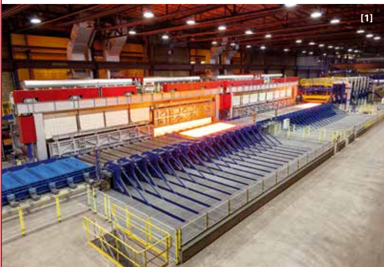
[1] | Two thermal treatment furnaces with [2] | directly linked quencher.
